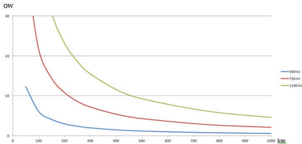
Figure 5 : Maximum transmissible power for typical OHL
